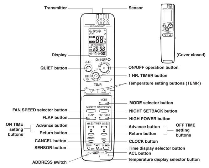
**NOTE** The illustration above pictures the remote controller after the cover has been opened.
